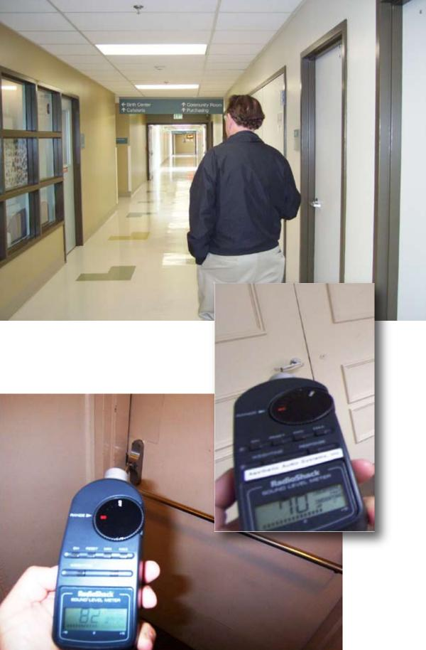
The doors measured 70+dB in many areas, with doors on closing registering over 80dB. Aesthetic Audio Systems (AAS) reported the challenging doors in an acoustic assessment report of findings. The doors were tuned and damped to reduce the slamming sound. Additionally, AAS created Harmonic Healthcare<sup>®</sup> music programs for specific areas of the hospital with the goal of relaxation in some areas, invigoration in others and patient nurturing in other areas.
